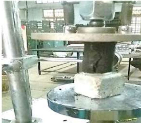
Fig 4 Testing Of Peat Soil Sample In Ucc Machine
